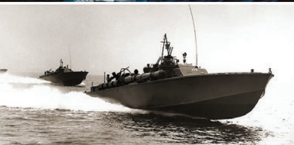
A PT boat built for speed and stealth could fire torpedoes at much larger ships. The Americans called them the "mosquito fleet." The Japanese called them "devil boats."
