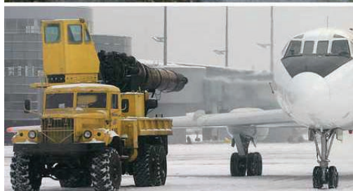
Russian snow blowers / dryers are armed with jet engines to blow away the snow and de-ice planes and runways.
